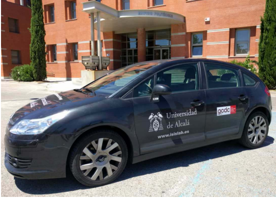
Fig. 1. University of Alcalá competition vehicle -DRIVERTIVE-: a modified fuel powered Citroën C4 with automatic transmission.
